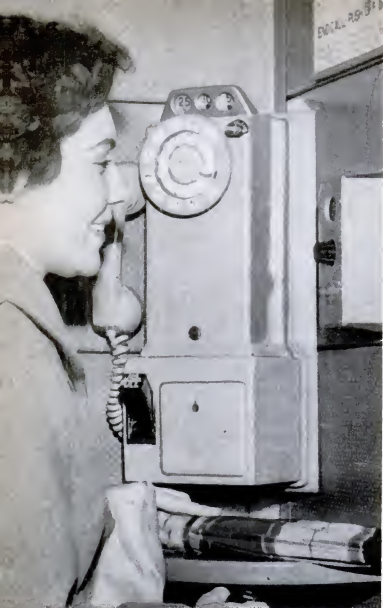
No-hands phone. Here's a phone you can talk into without taking it off the hook. The box at right is a combination mike and speaker for use by shoppers with arms loaded. Cincinnati is trying it.
